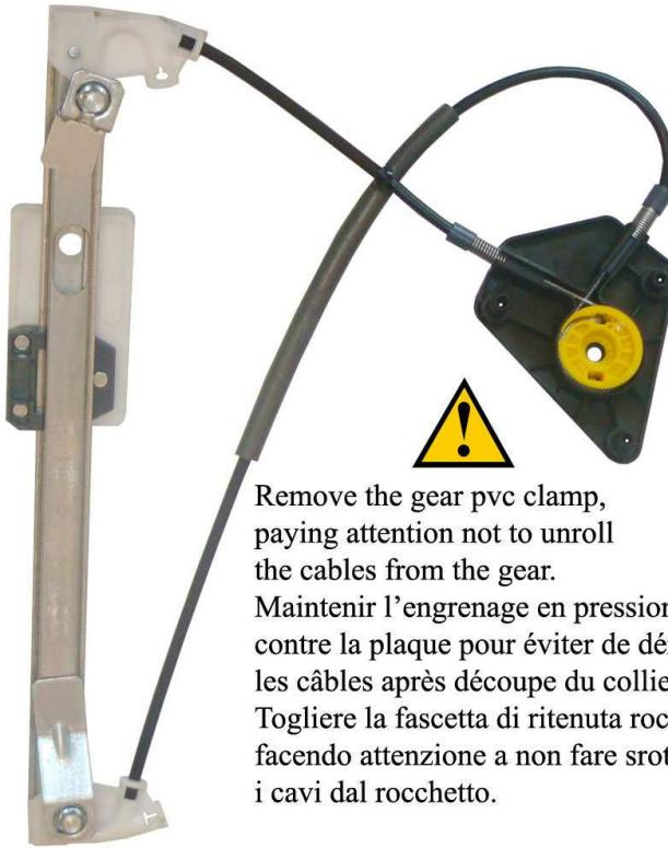
Remove the gear pvc clamp,
